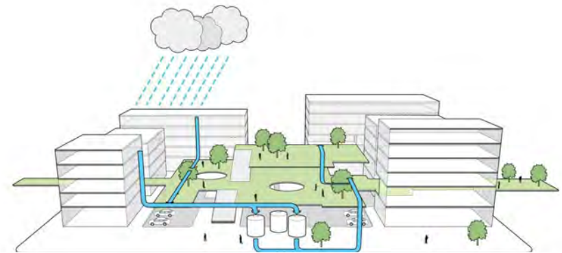
The terraced landscape between the buildings can filter water for use in grey water systems while excess run off is stored in at-grade tanks for future use.
